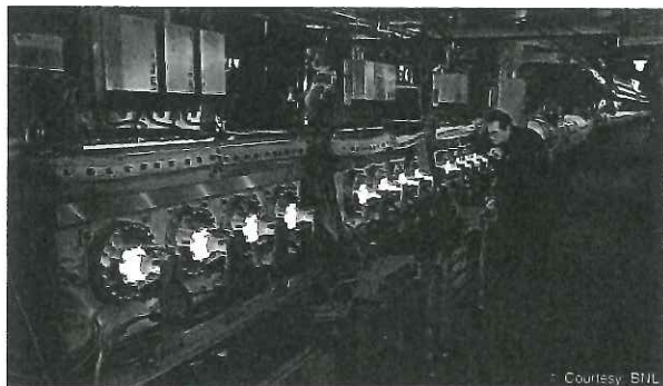
Technician Mike Myers checks components of stochastic cooling "kickers," which generate electric fields to nudge ions in RHIC's gold beams back into tightly packed bunches. This system of squeezing and cooling beams has produced dramatic increases in collision rates—and the data coming out of RHIC.
